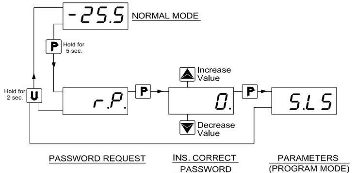
**Note:** If the Password gets lost, just swith off and on the instrument supply, push P key during the initial test and keeping the key pressed for 5 seconds.
