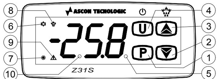
**1 - Key P** : Used for setting the Set point (press and release) and for programming the function parameters (hold pressed for 5 sec.)
