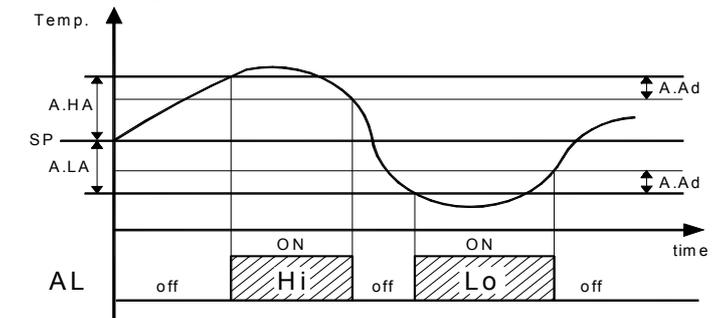
Temperature alarms of maximum and minimum can be disabled by setting the parameters "A.HA" and "A.LA" = oF.
